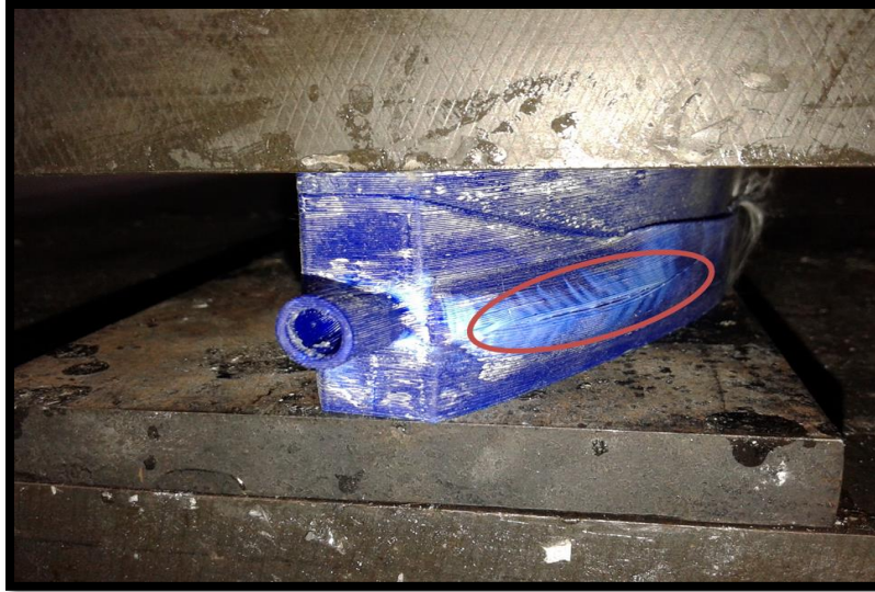
Fig. 39 Crack deformation in the sparse filled mold
