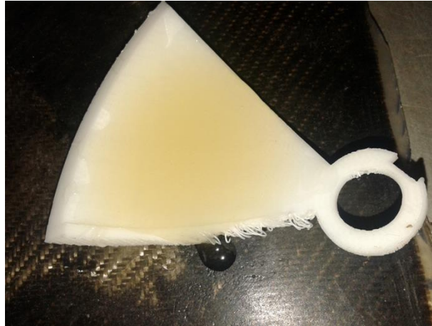
Fig. 33 FDM test specimen with epoxy resin
