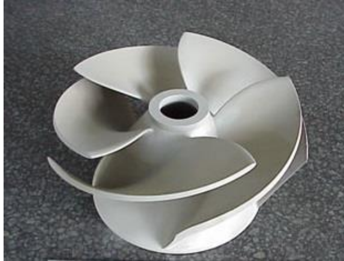
Fig. 5 Propeller made by SLS [13]
