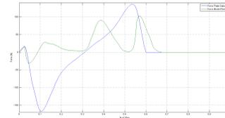
Figure 6: Comparison between the anterior/posterior component of the forces experimentally obtained with the ones calculated by the model.
