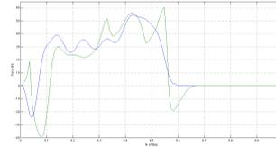
Figure 5: Comparison between the lateral/medial component of the forces experimentally obtained with the ones calculated by the model.
