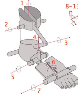
Figure 1: Representation of the axis of the degrees of freedom of foot model [5]
