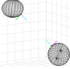
Figure 2: Representation of a pair of candidate contact points and their respective normal (blue), tangent (green) and binormal (magenta) vectors at the correspondent surface.
