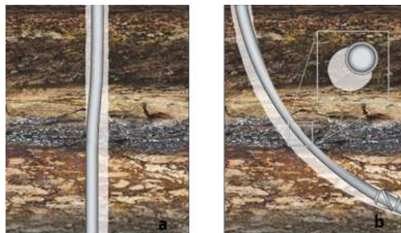
Figura 2.4 – Differential sticking (a) e Keyseating (b) (adaptada de Costo et al. , 2012).
