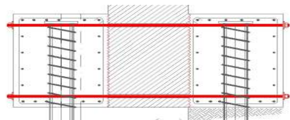
Figure 2 – Beams stabilizing the façade with the pre-stressed bar guaranteeing a better mobilization of the vertical loads (red) (adapted from [4])
