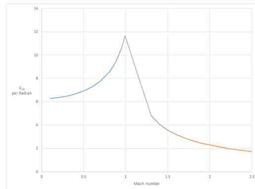
Figure 4: Lift-curve slope vs Mach number for the Box-wing forward 3D wing.
