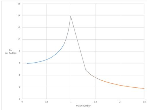
Figure 6: Lift-curve slope vs Mach number for the Utility 3D wing.
