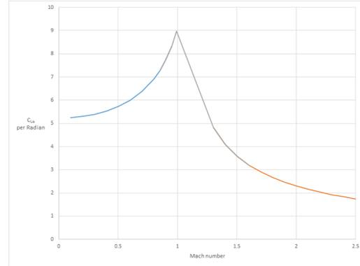
Figure 3: Lift-curve slope vs Mach number for the V-tail 3D wing.
