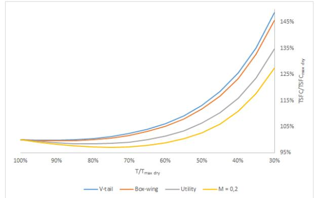
Figure 7: Part Power Operation for the three concepts cruise speed and for Mach = 0.2.
