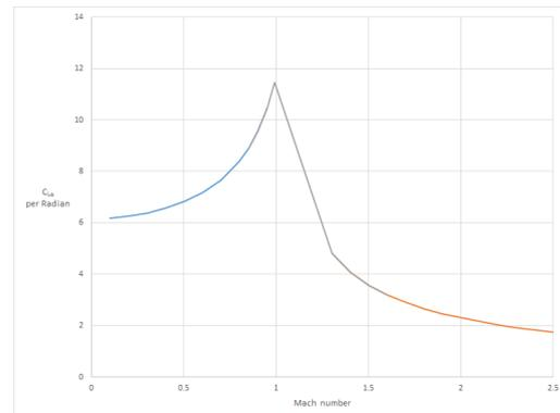
Figure 5: Lift-curve slope vs Mach number for the Box-wing afterward 3D wing.
