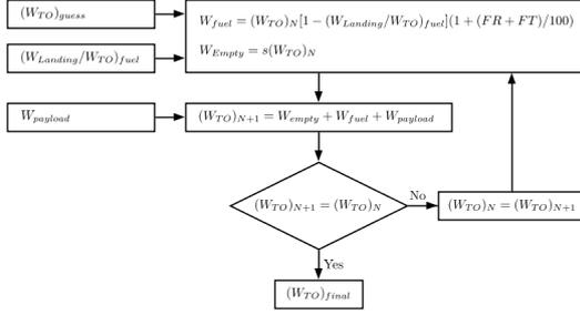
Figure 1: Algorithm for the calculation of the MTOW.
