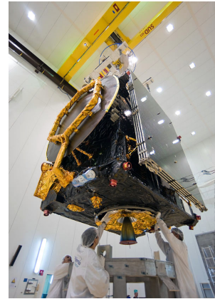
Figure 2: Thermal Deflector integrated on Spacebus 4000 at the base of Apogee Boost Motor (Source: ESA)
