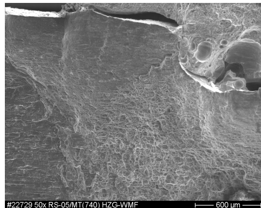
Figure 8: SEM: Crack extension and skin-stringer intersection
