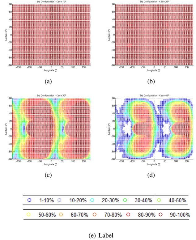
Fig. 1. Availability with the third configuration and (a) Cutoff angle of 10 degrees, (b) Cutoff angle of 20 degrees, (c) Cutoff angle of 30 degrees and (d) Cutoff angle of 40 degrees.
