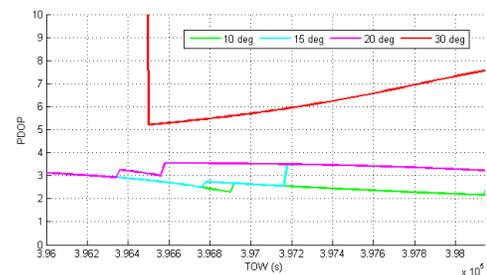
Fig. 6. PDOP values for Galileo-only positioning solution.
