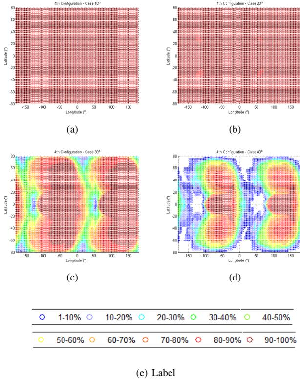
Fig. 2. Availability with the fourth configuration and (a) Cutoff angle of 10 degrees, (b) Cutoff angle of 20 degrees, (c) Cutoff angle of 30 degrees and (d) Cutoff angle of 40 degrees.
