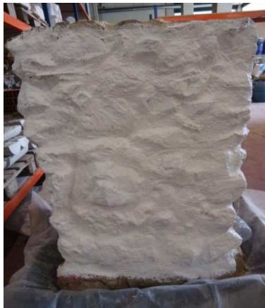
Fig. 15 – Rubber paint applied to the Surface "B".
