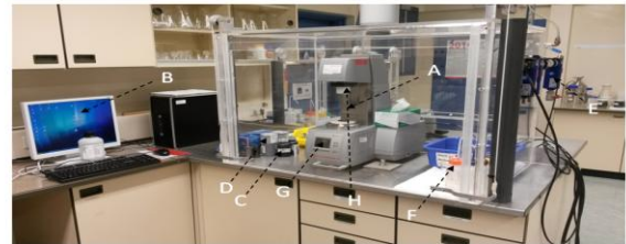
Figure 4: Experimental setup: A=mounting, B= computer with rheoplus software, C= sample from bioliq plant, D=spindle covering, E=pneumatic system for air pressure, F= methanol for cleaning, G= display of rheometer, H= covering to protect rheometer casing where spindle is attached
