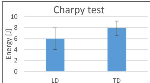
Figure 12 – The Charpy test results for heat treated specimens.
