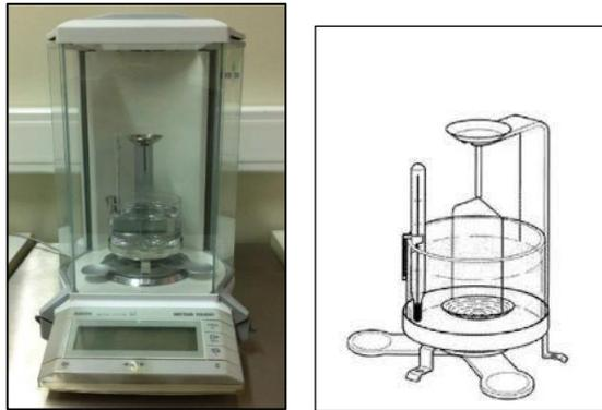
Figure 4 - Mettler AG 204 balance with the specific density measurement device.
