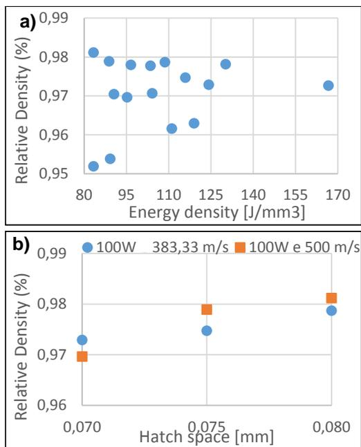
Figure 5 – a) Influence of energy density and b) hatch space on the relative density in the batch 1 results.
