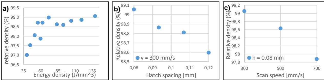
Figure 7 - Influence of a) energy density, b) hatch space and c) scan speed on the relative density in the batch 2 results.
