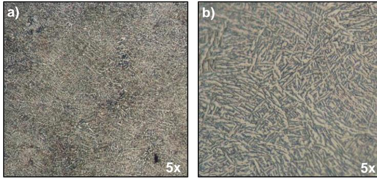
Figure 10 - Top view after heat treating at 900°C for 2h with furnace cooling. Lighter zones are  $\alpha$  phase and the dark zones are the  $\beta$  phase.
