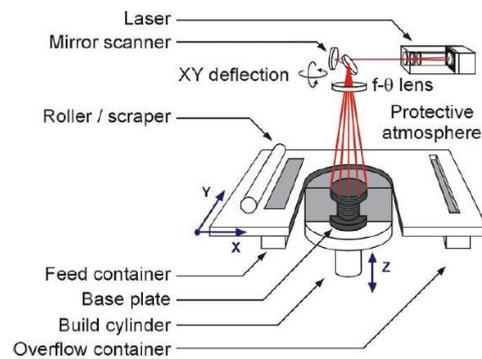
Figure 1 – Schematic view of SLM components [2].
