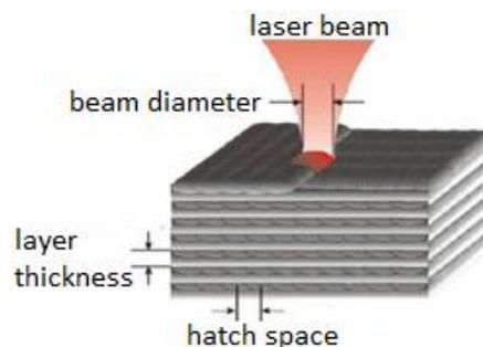
Figure 2 – SLM parameters (Image adapted from [11]).
