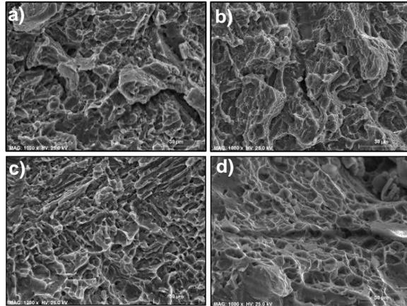
Figure 15 - Morphology of the fracture surface: a) 7\_3, b) 2a\_1, c) TT3 and d) TT7 specimens.
