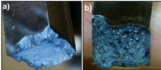
Figure 13 – USB Microscope images of heat treated specimens a) LD and b) TD.
