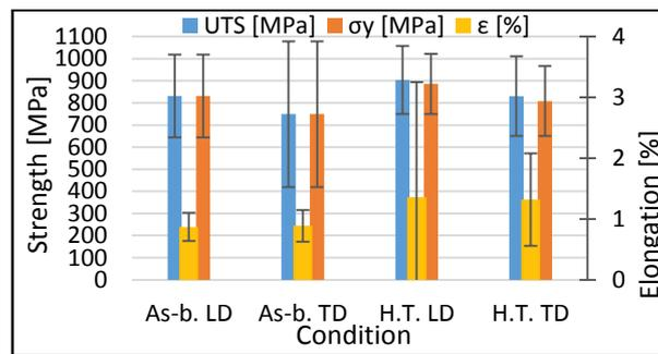
Figure 11 - Tension properties of as-fabricated and heat treated samples with different orientations.
