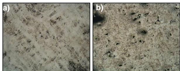
Figure 6 - Micrographs of SLM density specimens from batch 2: (a) top view of specimen 1 series 1 (99.09%), (b) top view of specimen 12 series 1 (97.49%).
