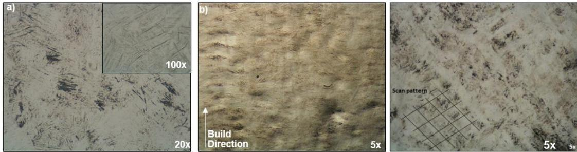
Figure 8 - (a) Top, (b) side view and (c) chessboard pattern in the top view of our untreated Ti6Al4V produced by SLM.
