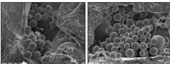
Figure 14 – SEM micrographs illustrating the present of defects.
