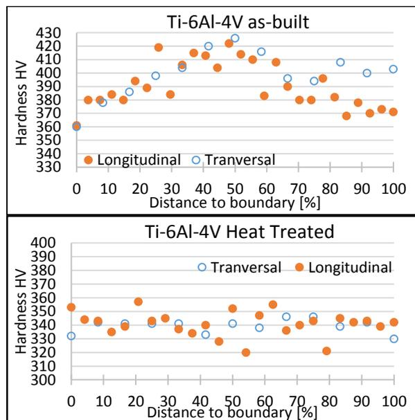
Figure 9 – Results of hardness analysis for as-built and heat treated samples.
