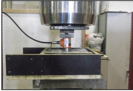
Figure 1 - Example of a punching shear test
