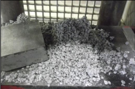
Figure 3 – BTC after compressive strength test
