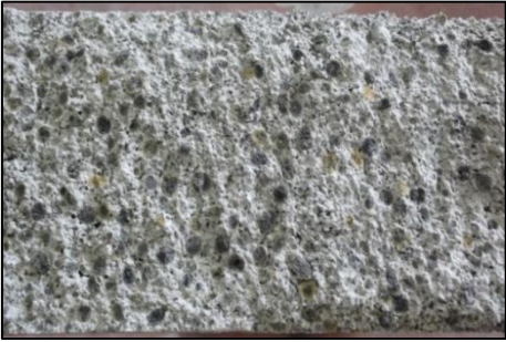
Figure 6 - Detail of the surface rupture (LUC) after tensile strength test
