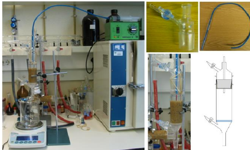
Absolute and effective permeability experimental apparatus in vertical direction
