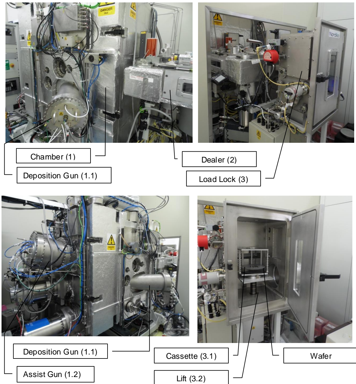
Figure 6 - Photographs of the N3600 at INESC-MN (taken at 19 of August 2014). a) Chamber, Dealer and Deposition Gun. b) Chamber showing the Assist Gun and the Cryogenic Pump. c) Load Lock and Dealer. d) Open Load Lock showing the placement of wafer on the Cassette.
