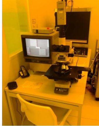
Figure 16 – Photographs taken in the yellow room of the Microscope Optical system (a bottom electrode defined by photoresist can be seen in the screen).
