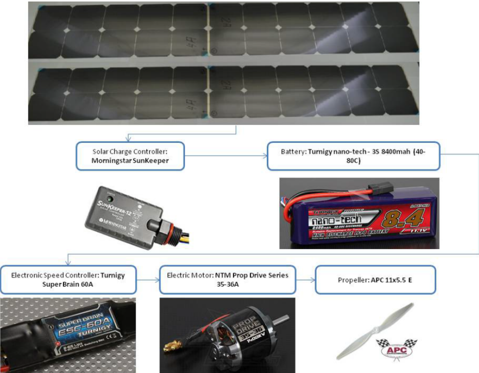
Figure 2.4: LEEUAV hybrid propulsive system scheme. [19]
