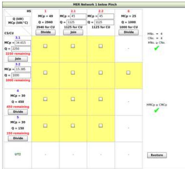
Figure 73 - Example 2 below PP MER Network 1 with stream division and non-equitable MCp values
