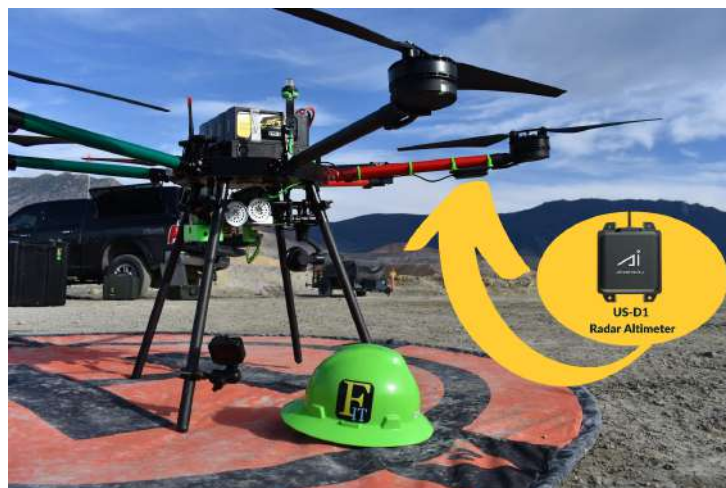
Figure 2.3: RADAR being used as altimeter [17]
