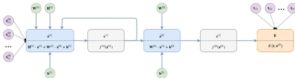
When one thinks about how to apply backpropagation to learn the parameters on such a network it may not seem obvious at first. However, if we unfold the network's function graph, the recurrent network becomes a much like a regular one.
