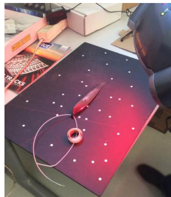
Figure 4: 3D scanning measurement of the blade
