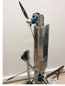
Figure 7: Resized support of the system motor+propeller
