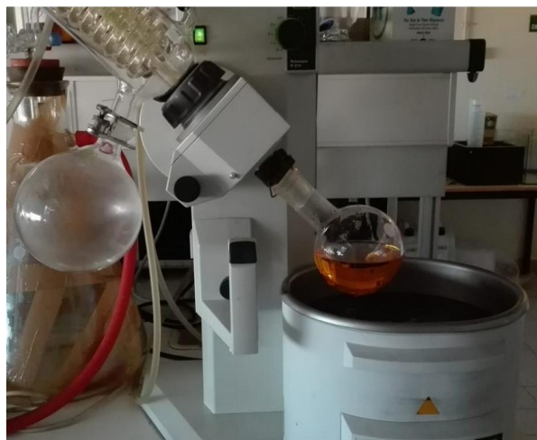
Figure 12 – Rotavapor® with reduced pressure used for oleic acid drying.
