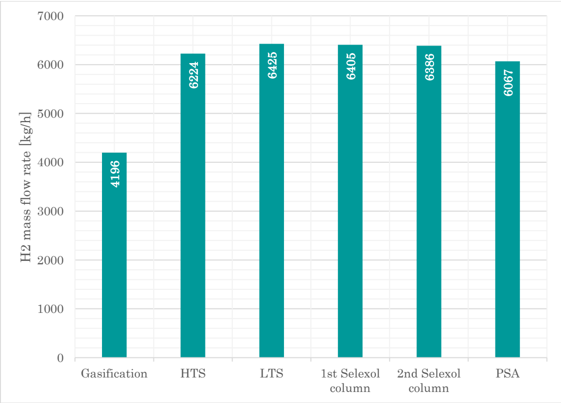
Figure 21. Mass flow rate of hydrogen after each process step based on Case 2.
