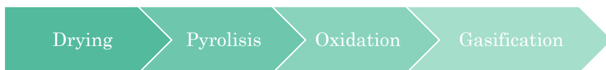
Figure 5. Process steps in gasification.
