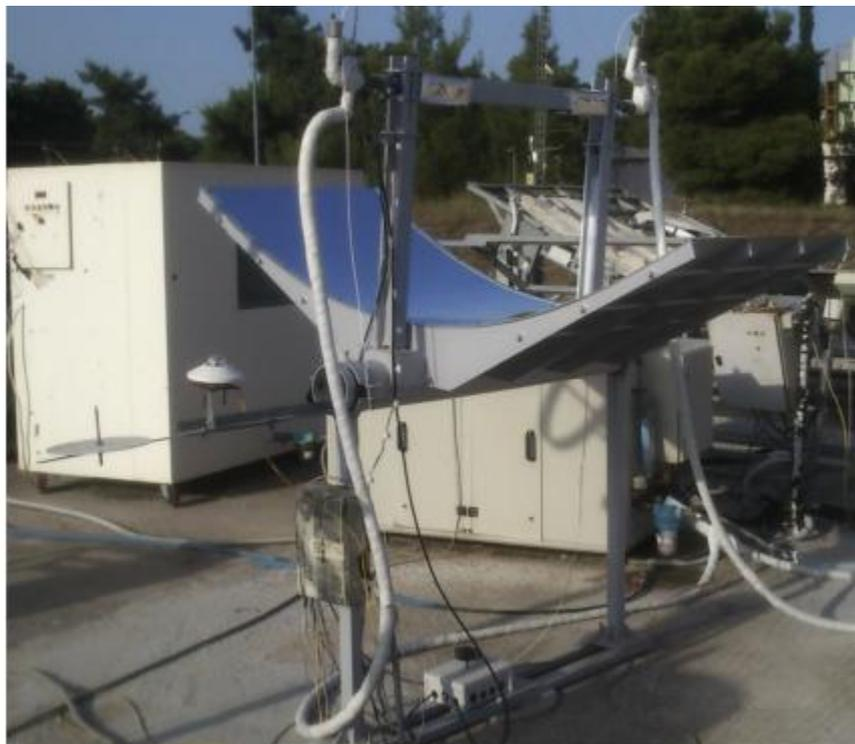
Figure 1. Prototype CPVT collector [6]
