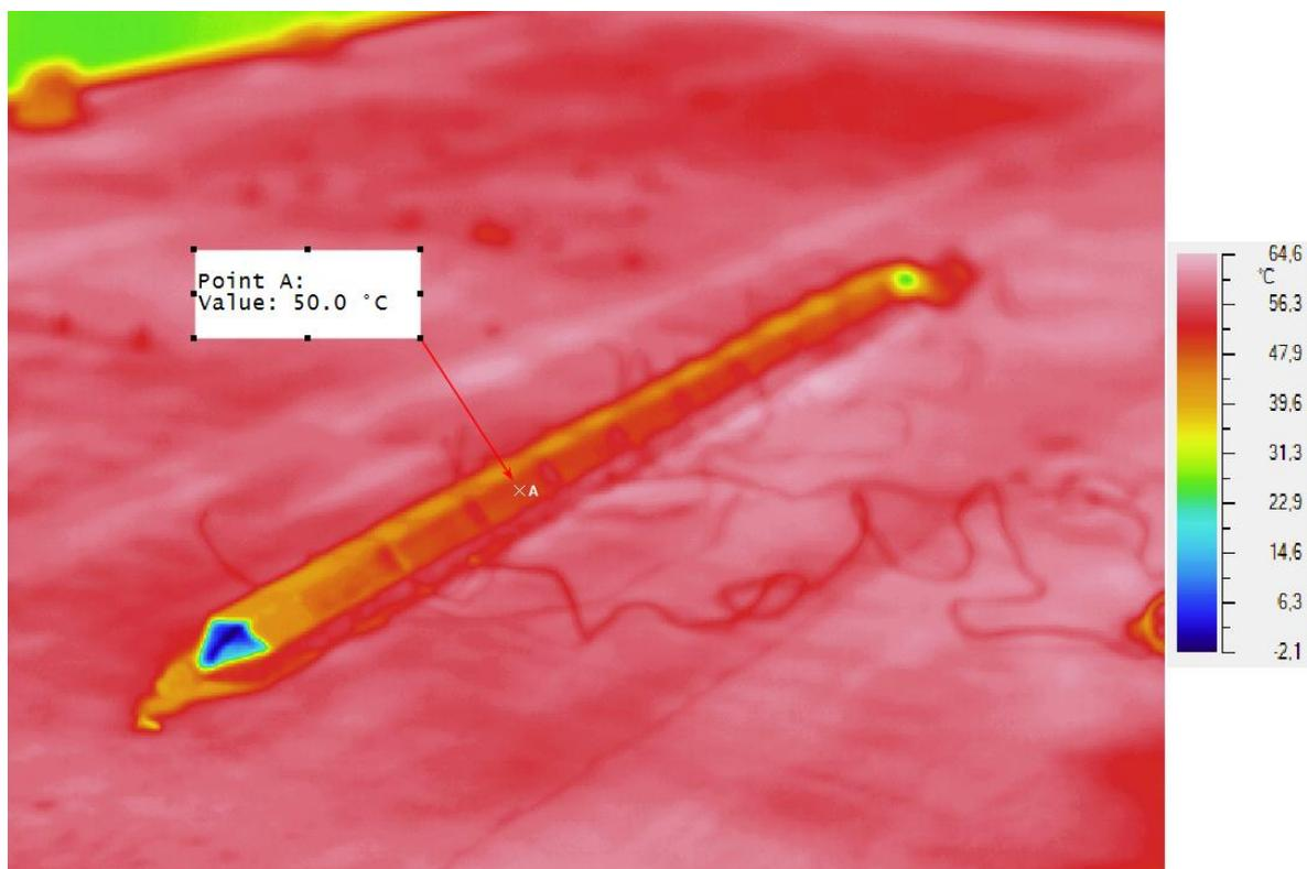
Figure 4. IR camera image – amorphous cells under 1 sun irradiance
