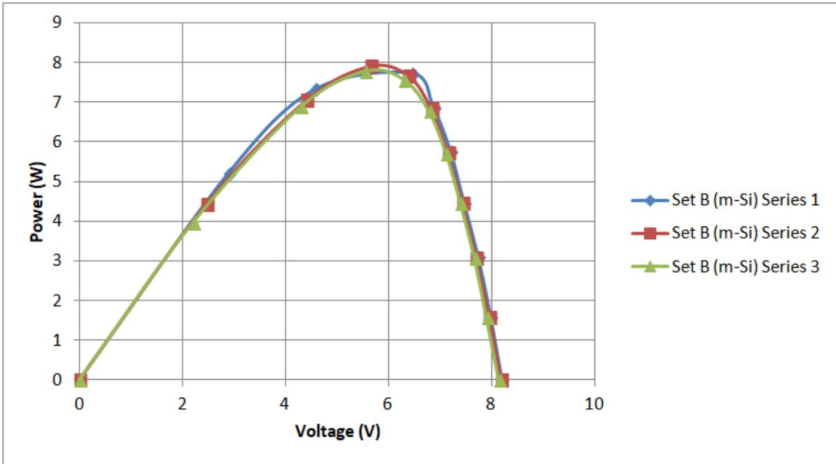
Figure 3. IV and power curves for Set B (m-si) under non-concentrated irradiance
