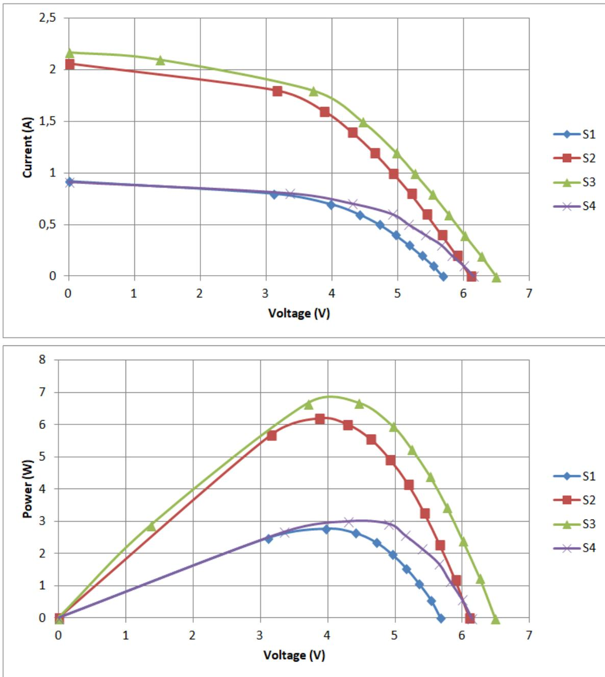
Figure 6. IV and power curves for chosen scenarios for Set A (a-si)
