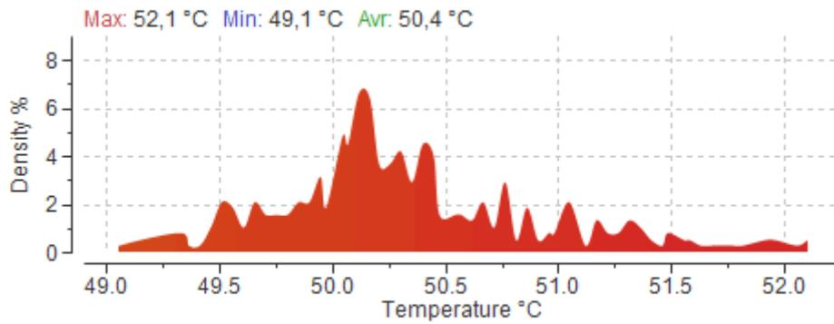
Figure 5. Temperature distribution for a-Si cells
