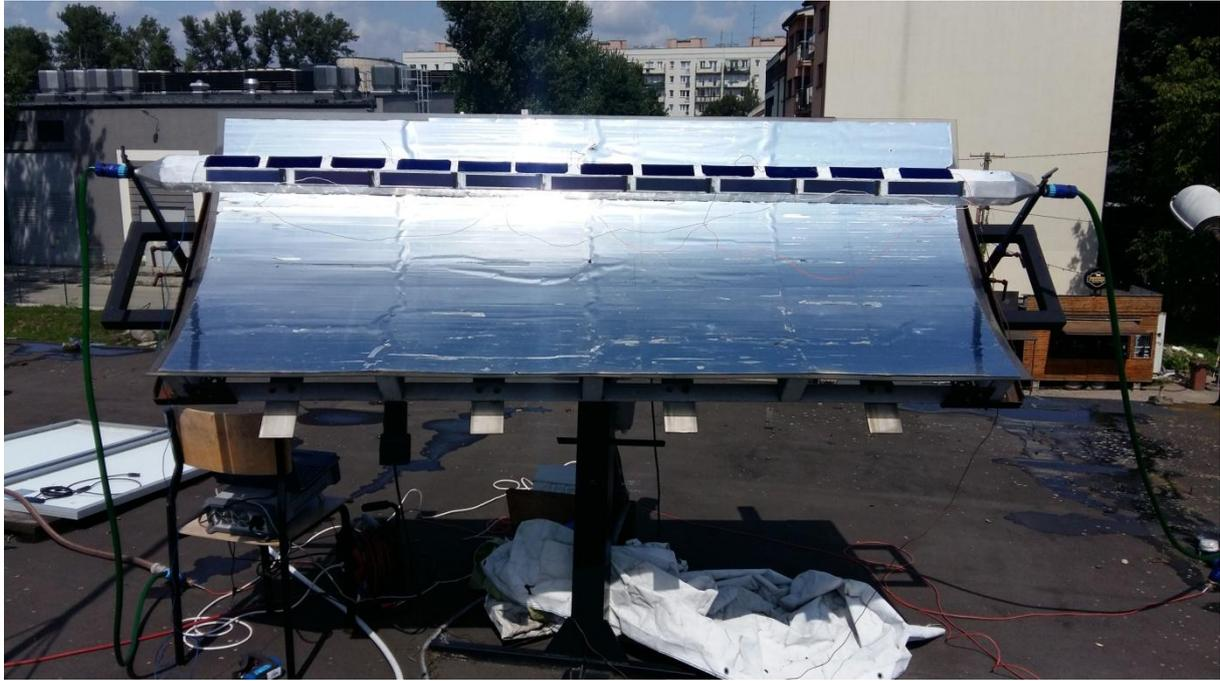
Figure 2. Fully assembled CPVT installation
