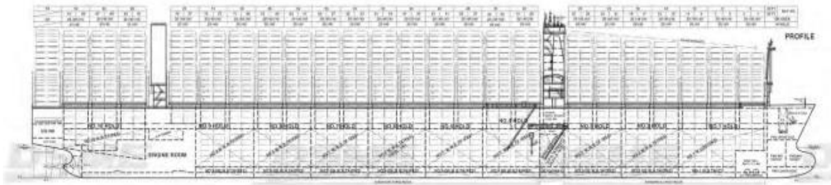
Figure 4.7 – Longitudinal cut of a malaccamax containership
