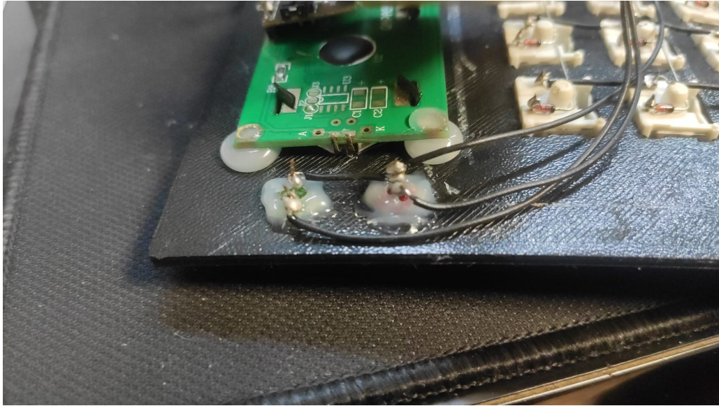
Figure 4.9: Example of some components that are glued to the enclosure.
