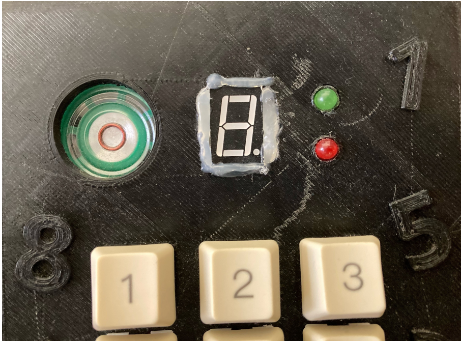
Figure 5.10: Damage sustained by the Simon Says interaction when attempting to widen the cutout 7-segment display cutout.
