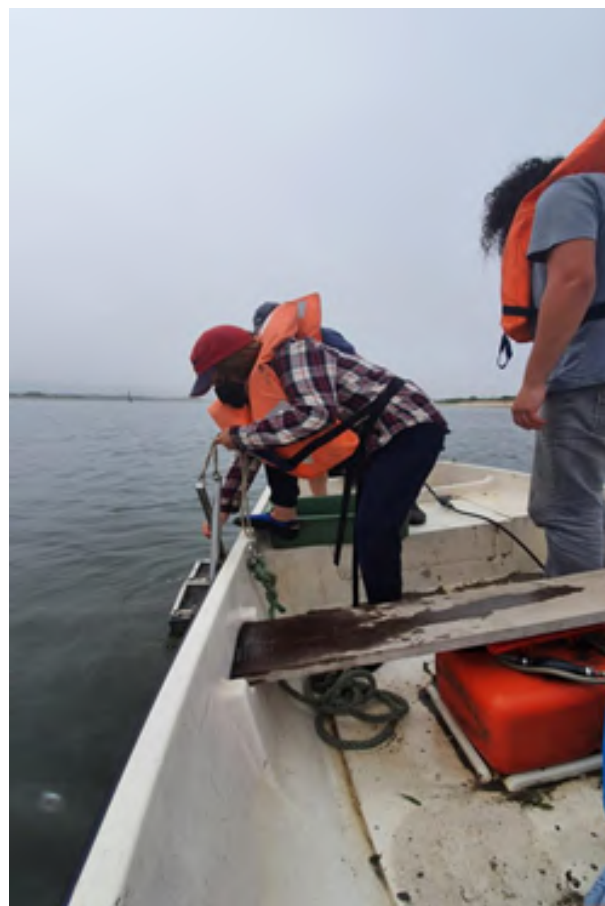
Figure 4.1: Sampling process during the field work, using a Van Venn dredge of 7 kg capacity.
