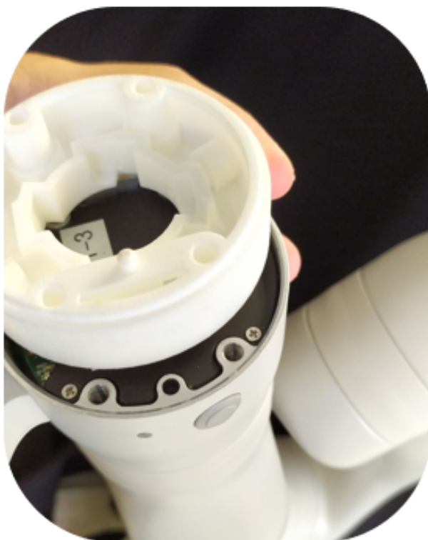
Figure 4.9: Adapter to couple the Seed Robotics hand to Kinova Gen3 arm
