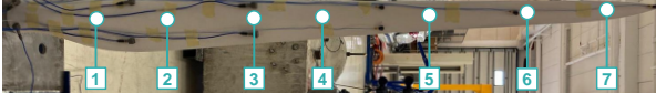
Figure 6: Mass positions used to perform the damaged experimental runs of the GFRP blade. between the experimental runs carried out with the GFRP blade in both healthy and damaged states.
