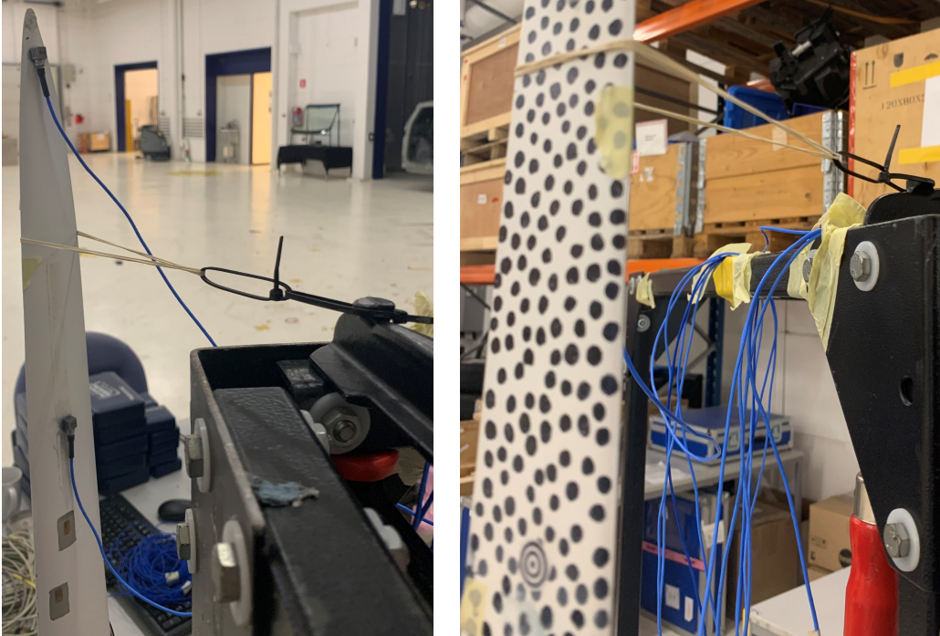
Figure 3.23: GFRP blade pull-and-release setup.
