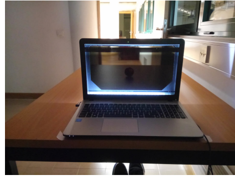
Figure 2. First Laptop successfully adapted into a transparent monitor .
