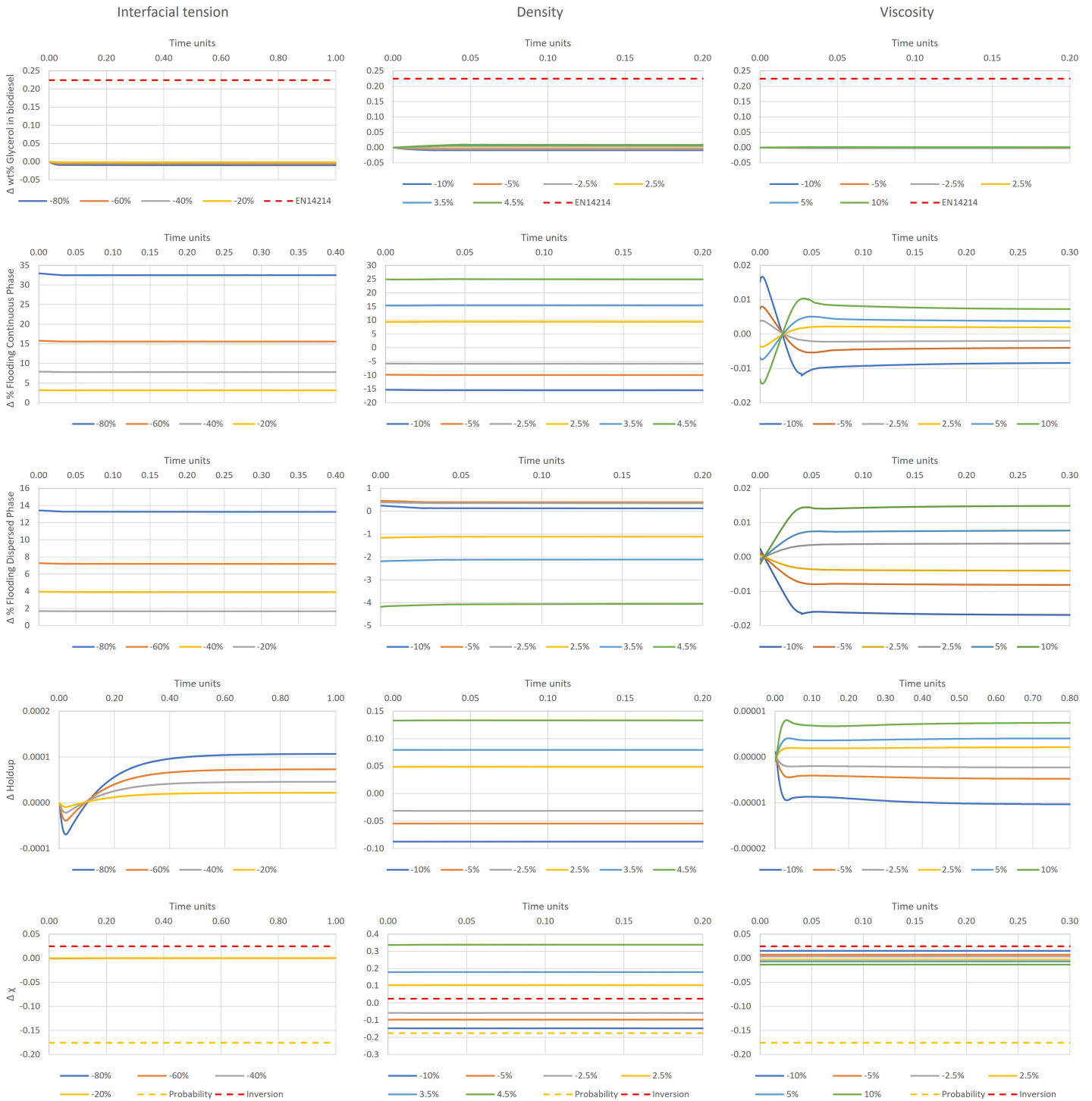
Figure 4.4: Open-loop testing for disturbances in interfacial tension, biodiesel density and biodiesel viscosity.
