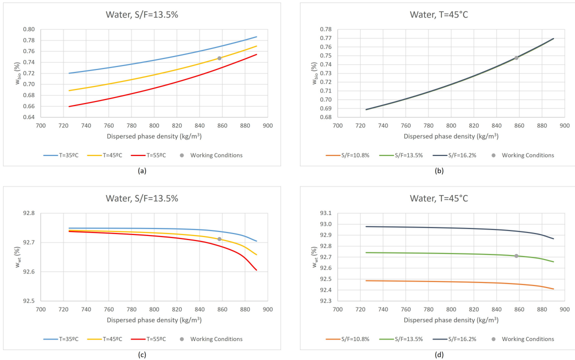
Figure 3.16: Impact of dispersed phase density in water solubility in biodiesel, (a) and (b), and in water, (c) and (d), for different solvent to feed ratios and temperatures with biodiesel inlet mass flowrate of reference.
