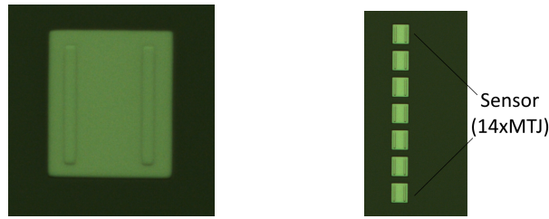
Figure 5.11: Individual Junction (Left) and Sensor Overview (Right) after the Bottom Definition Process
