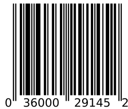
Figure 1.1: Typical example of a UPC-A Type Barcode (12-digit barcodes used in product tracking in stores and commerce - typical dimensions 3.73cm \times 2.59cm^2 )
