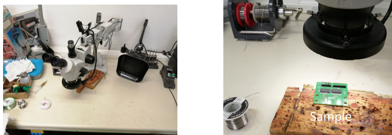
Figure 6.3: Soldering Station (Left) and the Soldering of the Sample (Right)
