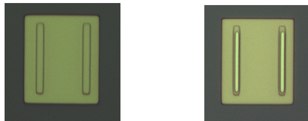
Figure 5.12: Closed Junction (Left) and Opened Junction (Right) after the Vias Opening Process
