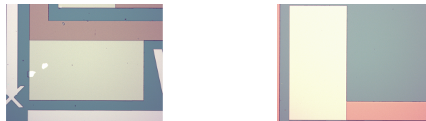
Figure 5.14: Ground Pad (Left) and Positive Pad (Right) after the Pad Opening Process
