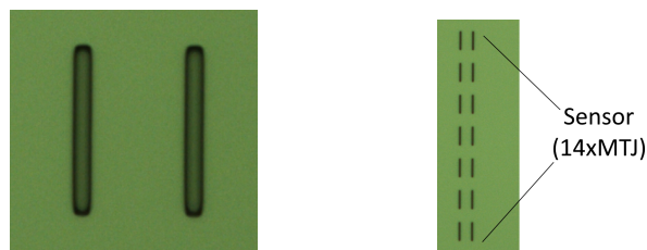
Figure 5.10: Individual Junction (Left) and Sensor Overview (Right) after the Pillar Definition Process
