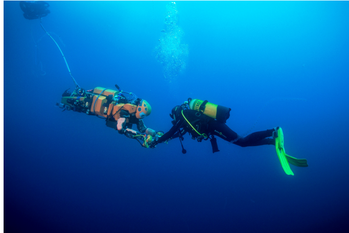
Figure 1.3: Ocean One diving in the Mediterranean at 15 m, interacting with the diver in a compliant and safe manner (obtained from ) [23]).
