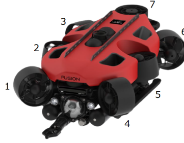
Figure 6.1: Perspective of the FUSION vehicle and identification of its seven thrusters. (source: https://www.srsfusion.com/srs-fusion )
