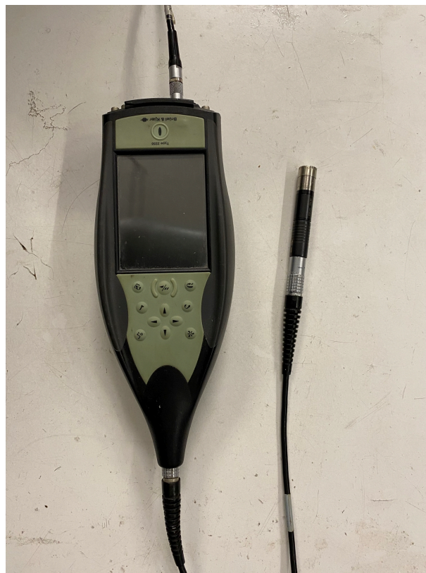
Figure 2.5: Microphone system used for capturing the frequencies and sound pressure level of the sound emitted by the instabilities.
