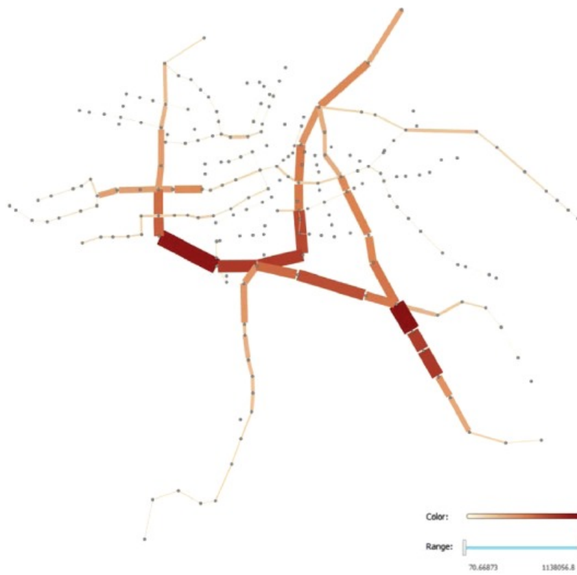
Figure 3.6: Link criticality indicator in Cats et al. [9] robustness assessment during a disruption scenario.
