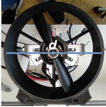
Fig. 18. Ducted fan with the propeller installed. d is the ducted fan diameter.
