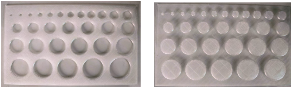
Figure 3.35: Dimensional test plate with holes (left) and cylinders (right)
