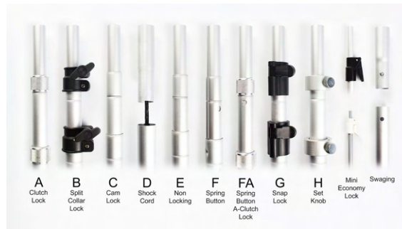
Figure 3.22: Various types of telescopic locks available in the market [98]
