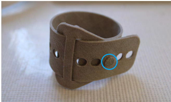
(a) 3D printed TPU strap
