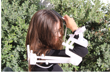
Figure 5: 3D printed prototype of the exoskeleton being used while performing the ADL of brushing hair
