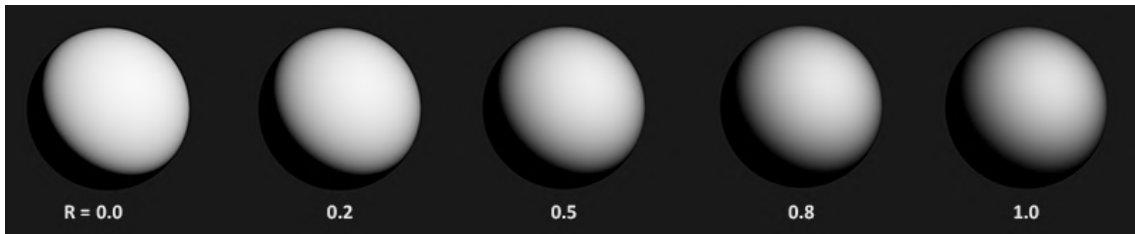
Figure 4.7: GGX Geometry. Roughness values. (Source: Joey de Vries [31])
