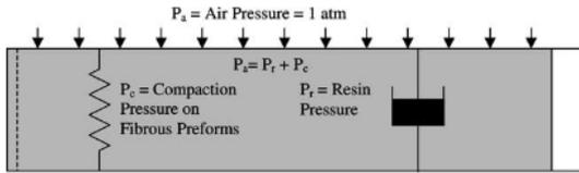
Figure 2: Pressure distribution inside the mould, [11].
