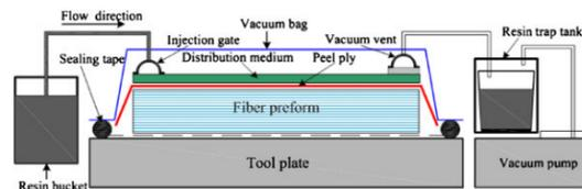
Figure 1: VI setup components, [2].
