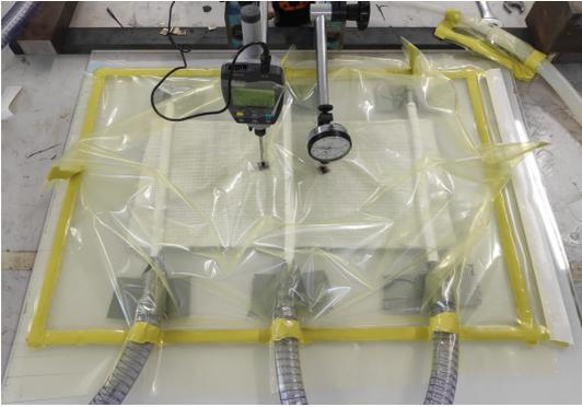
Figure 3: Setup for material characterisation tests.
