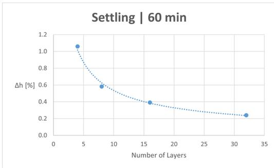
Figure 5: Thickness variation during settling stage.
