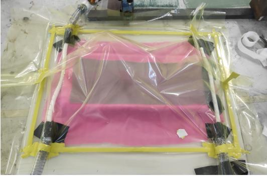
Figure 7: Setup for infusion tests.
