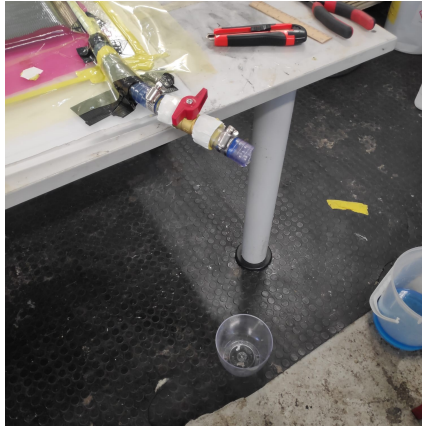
Figure 4.25: Resin inlet hose cut after the filling stage.
