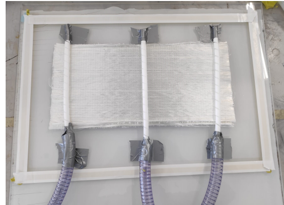
(b) Step 4: Resin inlet and outlet.
