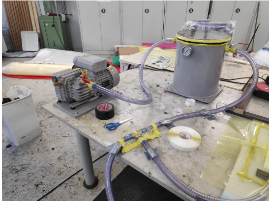
(a) Hoses from setup to vacuum pump.
