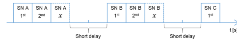
Figure 18: Representation of a short delay between the time slots of SNs to ensure that there is no overlapping between them in case of x attempted failed communications, x being the maximum number of attempts within a set period of time.
