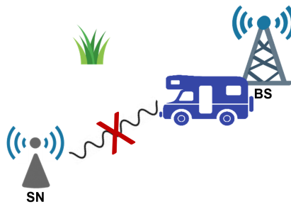
Figure 5.9: Unexpected obstacle in the sensor node's radio path to the base station, which blocks the communication signal (this image was designed using resources from [3–5]).
