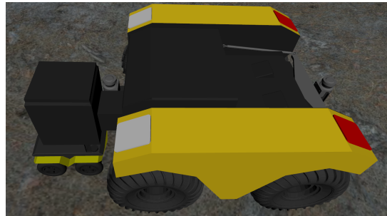
Figure 6.11: Jackal coupled to the Warthog to simulate recharging;
