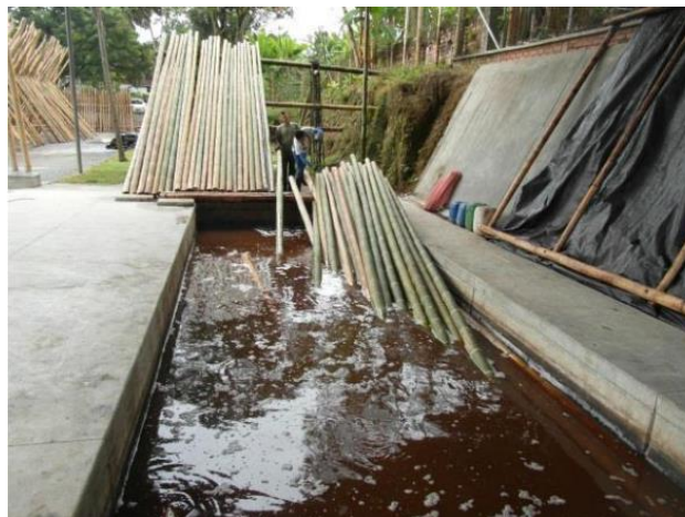
Figure 15- Bath/Soaking method using boron, Colombia (Kaminski et al., 2016)
