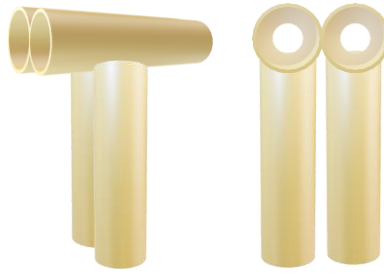
Figure 50- Illustration of a possible solution to avoid shear forces in the centre beam of the floor.
