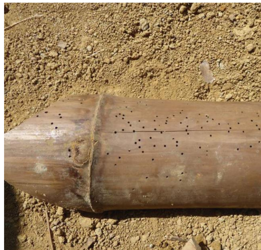
Figure 12- Beetle exit holes visible inside of bamboo (Kaminski, 2018).
