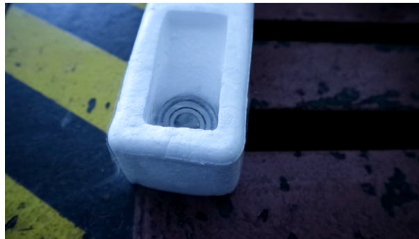
Figure 4.9: Bearing cryogenic test
