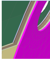
Figure 14: Example of the laminate offset, with an aluminium part in pink, and the layers of the composite aligned
