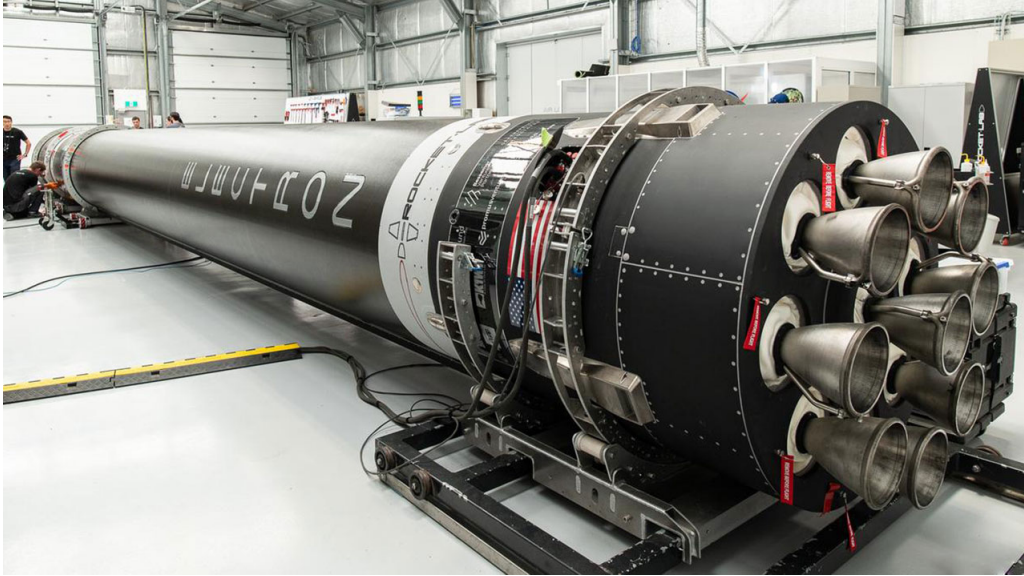
Figure 2.2: Rocket Lab Electron made of carbon-composite fiber
