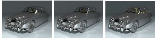
Figure 3: MLT (left), BPT (middle) and PPM(right) outputs of the same scene.(Source:Georgiev 2012 [4])
