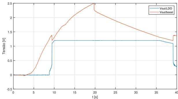
Fig. 10. Time diagram for the analysis of the influence of the super-capacitor in the final prototype with  $R_L = 100 \text{ k}\Omega$ , when the input voltage is given by the TEG. Observing the voltage at the output of the *boost* converter and the LDO.
