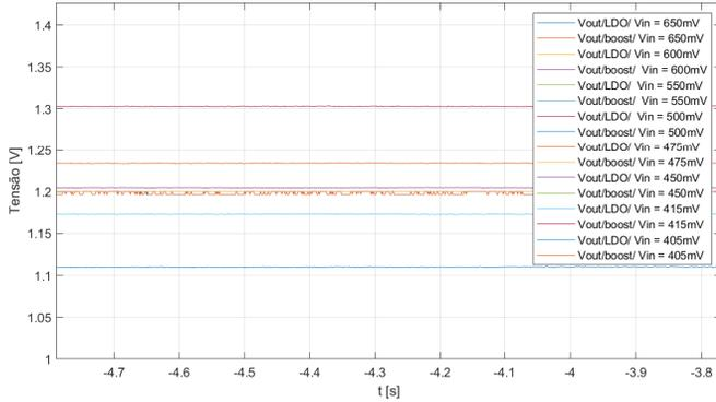
Fig. 9. Time diagram for the analysis of the influence of the input voltage on the output voltage of the LDO.
