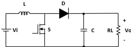
Fig. 2. Schematic of the Step-up DC-DC Converter.
