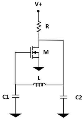
Fig. 4. Schematic of Colpitts LC oscillator.
