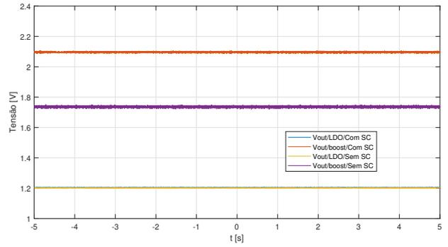
Fig. 7. Time diagram for the two final prototype cases, with and without super-capacitor. Being the circuit fed by an ideal input voltage of 0.5V, with  $R_L = 100k\Omega$  and observing the voltage at the output of the converter boost and at the LDO output for both cases.
