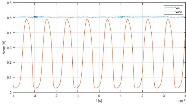
Fig. 5. Waveform resulting from the experimental setup, on the test board, of Colpitts LC oscillator for an input voltage of 0.5 V.
