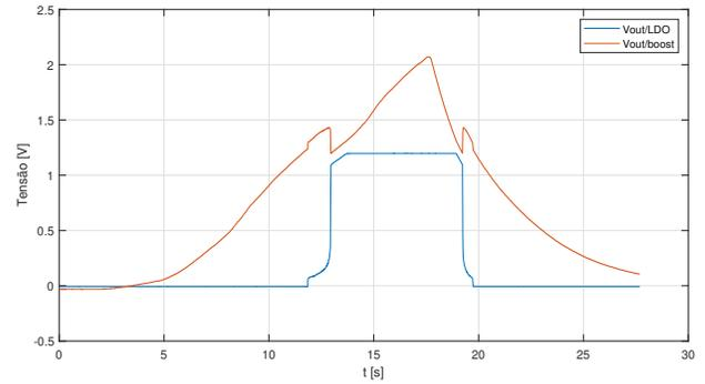
Fig. 11. Time diagram for the analysis of the influence without super-capacitor in the final prototype with  $R_L = 100 \text{ k}\Omega$ , when the input voltage is given by the TEG. Observing the voltage at the output of the *boost* converter and the LDO.
