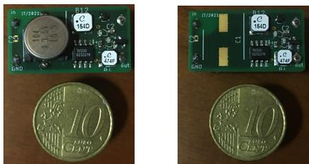
Fig. 6. Final prototype of the *boost* converter with (left) and without (right) super-capacitor.
