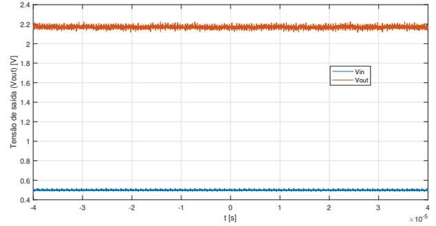
Fig. 3. Time diagram of the output voltage of the Step-up DC-DC Converter (orange) for  $V_{in} = 0.5 \text{ V}$  (blue),  $f_c = 1 \text{ MHz}$ ,  $D = 50\%$ .
