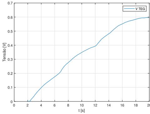
Fig. 1. Variation of TEG Voltage with time, while heating TEG, with initial temperature of 25°C and final temperature in the hot side of 230°C.
