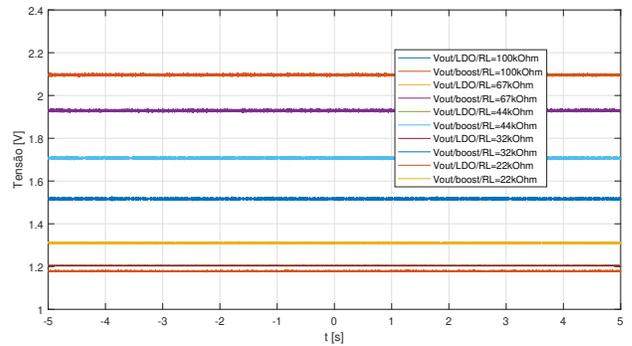
Fig. 8. Time diagram for the analysis of the influence of the load resistance  $R_L$  in the final prototype with super-capacitor. Being the circuit fed by an ideal input voltage of 0.5V and observing the voltage at the output of the converter *boost* and the LDO.
