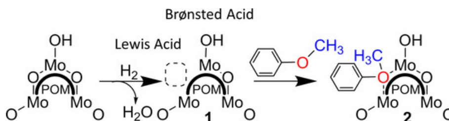
Figure 13: Representation of surface reduction, step 1, and reactant adsorption, step 2.
